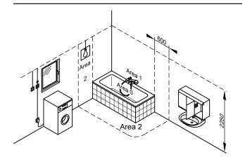
Electrical equipment in rooms containing a bathtub or a shower must be installed in such a way that users cannot be exposed to dangerous body currents.
