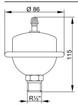
If the pipework to which the Vitodens is connected also supplies draw-off points at which water hammers may occur (e.g. pressure washers, washing machines or dishwashers): Install shock arrestors near the source of the water hammer (recommended).
